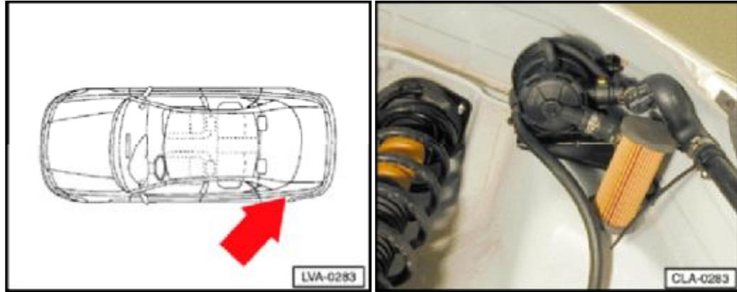
**V144 Leak detection pump (LDP)**
