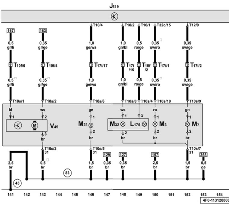
**Onboard supply control unit, right headlight**
